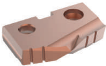
150° Structural Steel For material over 7/16" thick and for reduced exit burr
