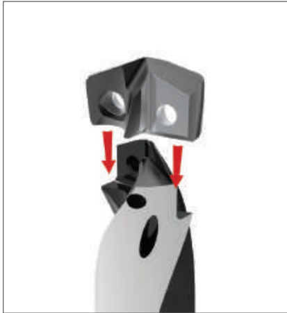
Step 1: Align the flats on the GEN3SYS XT insert with the flats on the ears of the holder.
